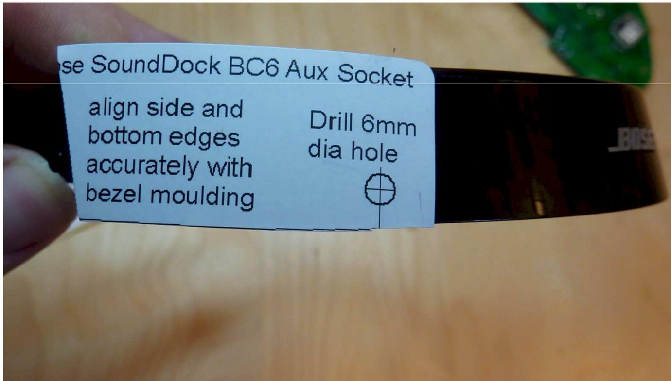
Drill small pilot hole. Align drill vertically to curved surface in line with an imaginary line pointing at the centre of the curve. In the other plane align drill parallel to the base of the dock. Make sure the centre of the drill aligns with the cross-hairs inside the circle.
